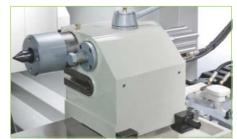
(F) Hydraulic tailstock with manual movement
